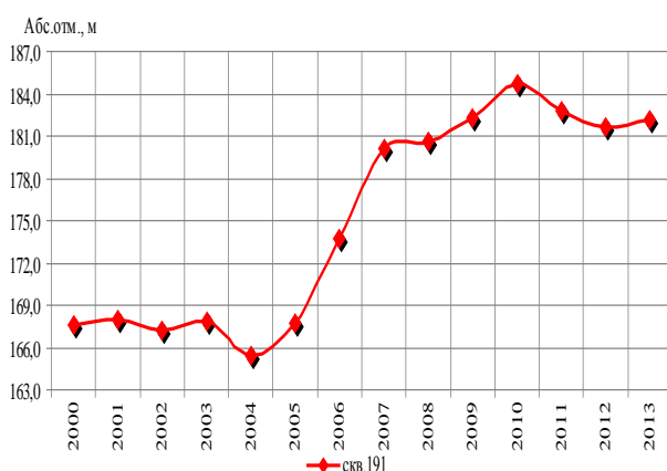
Picture 1 – Diagram of ground water levels changing in observation well № 191 of “Novinki” intake
