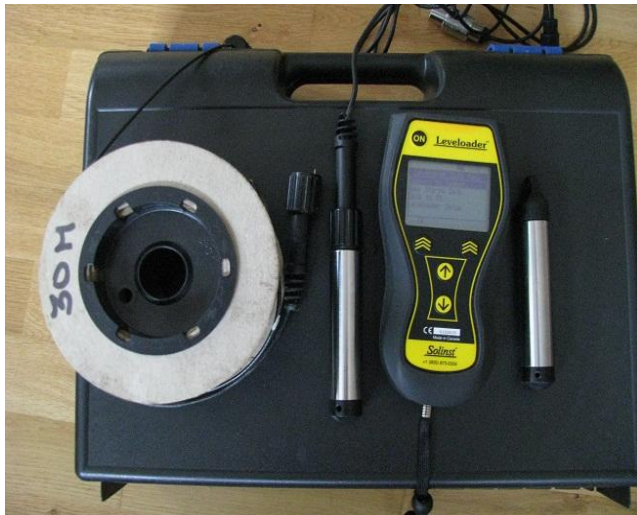
Automatic water level meters
